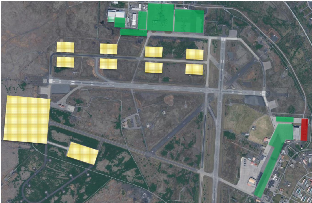
Figure 2. Apron priorities. The green areas are serviced on a daily basis. The yellow ones are serviced on demand in collaboration with APOC and The Coast Guard. The aircraft stands in red east of hangar 885 are closed during winter.
